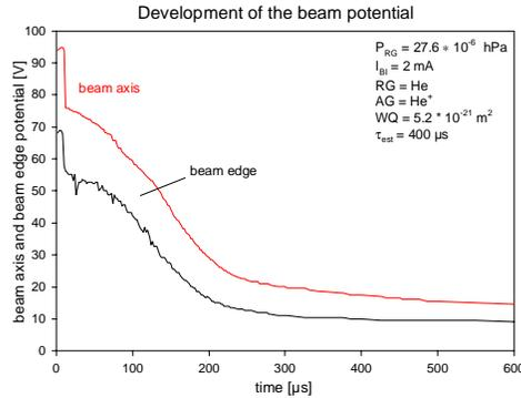
Figure 4: Temporal development of beam potential
